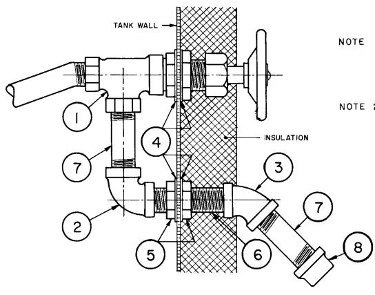
NOTE | THE SAMPLING VALVE SHALL BE MOUNTED IN THE LOWER HALF OF THE REAR BULK HEAD, AT LEAST 300 mm FROM THE SHELL. THE VALVE CONTROL AND THE OUTLET SHALL BE LOCATED SO AS TO PERMIT SAFE AND CONVENIENT OPERATION AND SAMPLE GATHERING.
