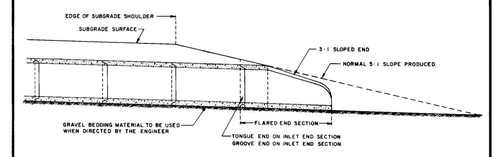
NOTE: I. BACKFILL UNDER PIPE HAUNCHES AND IMMEDIATELY ADJACENT TO PIPE TO BE PLACED IN LAYERS NOT EXCEEDING 150mm and Thoroughly COMPACTED AT OPTIMUM MOISTURE WITH PNEUMATIC OR OTHER MECHANICAL TAMPING EQUIPMENT.
