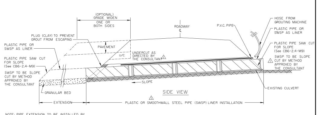
NOTE: PIPE EXTENSION TO BE INSTALLED BY CONVENTIONAL METHOD (AS DETERMINED BY THE CONSULTANT)
