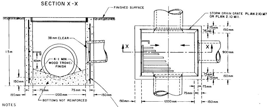
STEEL LADDER RUNGS TO BE INSTALLED AT 40 cm INTERVALS
