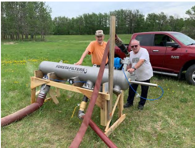
Gull Lake Watershed Society members testing a smaller scale Forsta pressurized filter.
